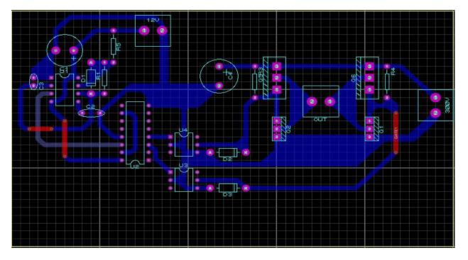
While making PCB layout we tackle many difficulties. The main difficulty is to arrange component in PCB. Make sure that no wire is left unconnected or shortcircuited. And try to make as compact as possible.
